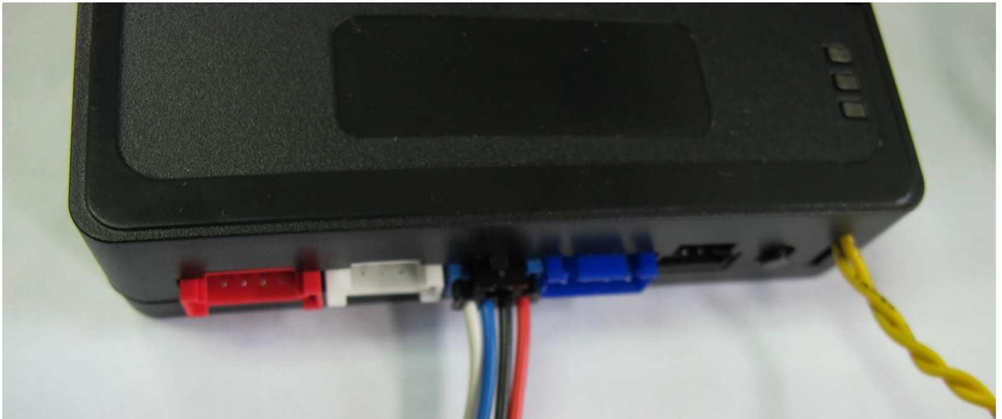
9. To program the Text2Car on the EVO-ONE, Turn IGNITION ON. Press and hold Valet switch until the side red light flash on EVO-ONE then release. Press and release the Valet switch 5 times. Press and release the Brake pedal once. Send lock with Text2Car interface. Turn IGNITION OFF.
